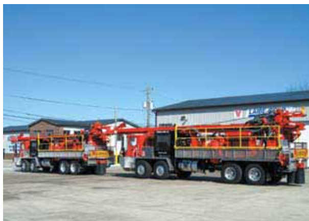
Bunbury Drilling of Bunbury Western Australia takes delivery of two new V-2095EXP rigs, equipped with 1,250/350 air compressors, 3-by-4 centrifugal mud pumps, 95,000 pounds standard pullback, and mounted on a 6-by-8 carriers with CAT C18 diesel engines.
